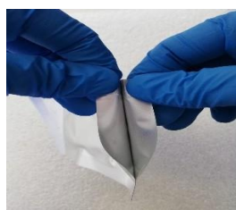
External Casing Opening : remove each corner first, one by one
